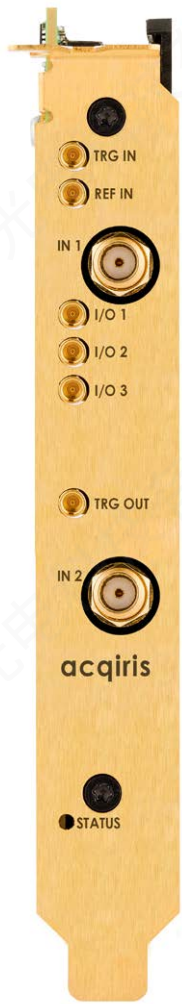
Figure 3. SA240P front panel, with analog inputs and multiple programmable I/O signals.
