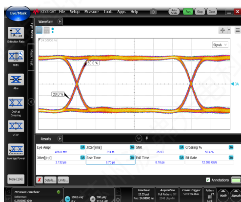
Input signal Eye amplitude = 0.45 \text{ V}_{\text{pp}}
