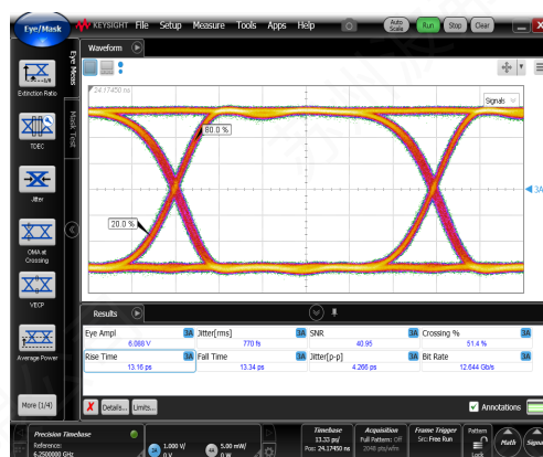
Output response Eye amplitude = 6 \text{ V}_{\text{pp}}
